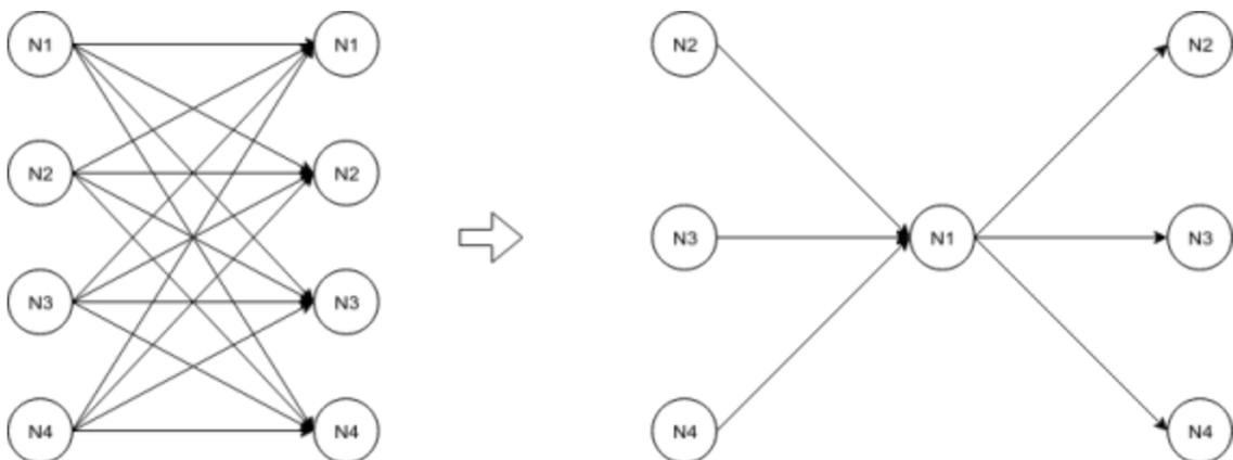
Figure 3. BFT's mesh vs. HotStuff's Star network
